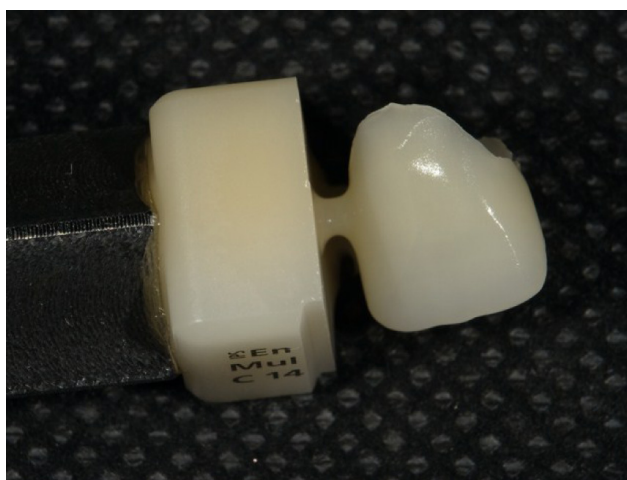
Figure 6: Empress CAD multi block, after removal from the milling machine.
