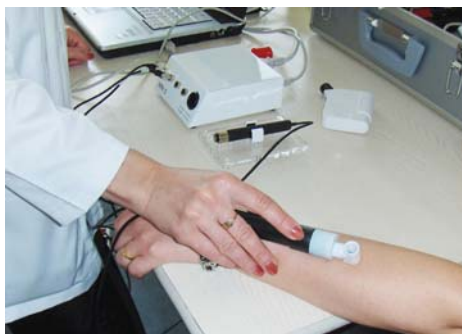
Figure 1. Measurement of transepidermal water loss by Tewameter® TM 300 and Multi Probe Adapter Systems® (product of Courage+Khazaka, Germany).
